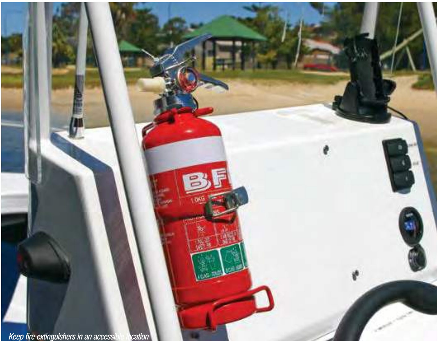
Check the gauge is in the green
